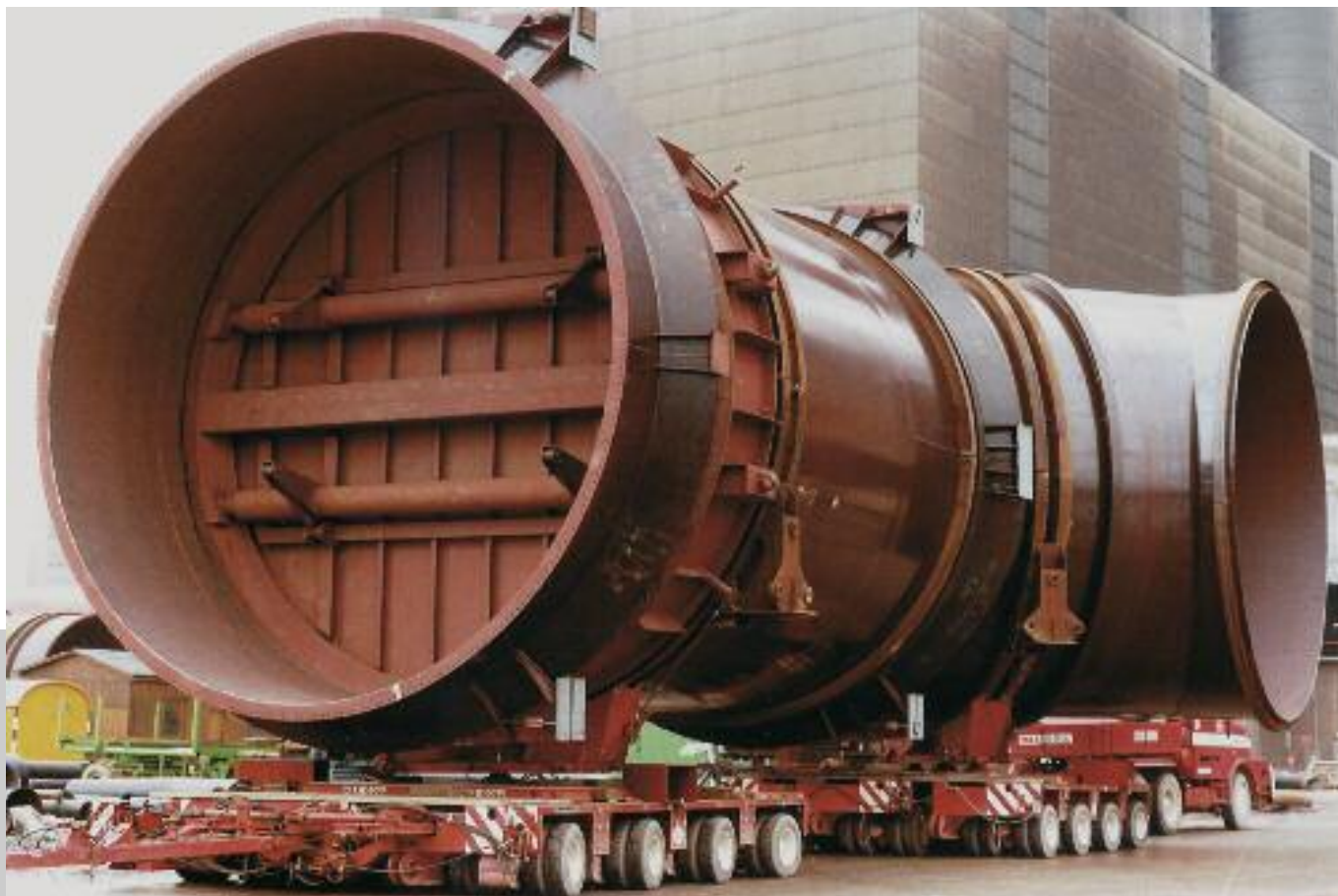
Illustration below: Two gas dampers NS 7480x5300 mm for the DeNOx plant at the AMER power station in Holland at the Rauenstein works. Completion with the duct piece takes place on-site.
