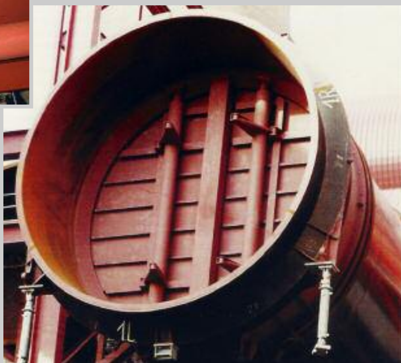
Illustration above: Flap damper NS 7480 x 5300 mm. Supplied for the De-NOx plant at the AMER power station in Holland. The lattice supported blade is driven via a toggle system (insert). 100% gas-tight using the NICROFLEX-HIPERFORM sealing system.
