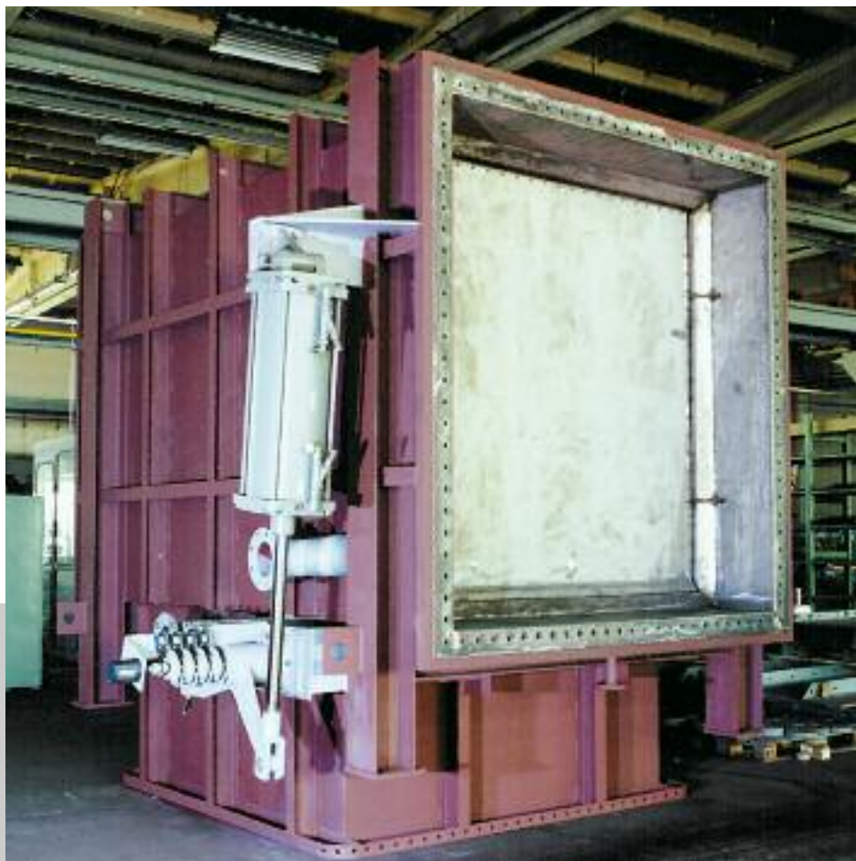
Gas diverter 4800 x 5300 mm, supplied for the FDG at the WESER power station, Veltheim BRD. Built-in scrubber. Drive via toggle. With double sealing and purge air, 100% leak-tight shut-off.
