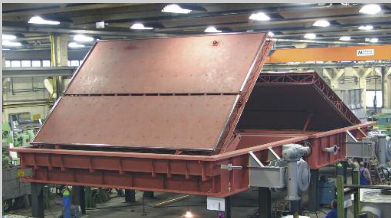
Illustration below: Two gas dampers NS 7480x5300 mm for the DeNOx plant at the AMER power station in Holland at the Rauenstein works. Completion with the duct piece takes place on-site.
