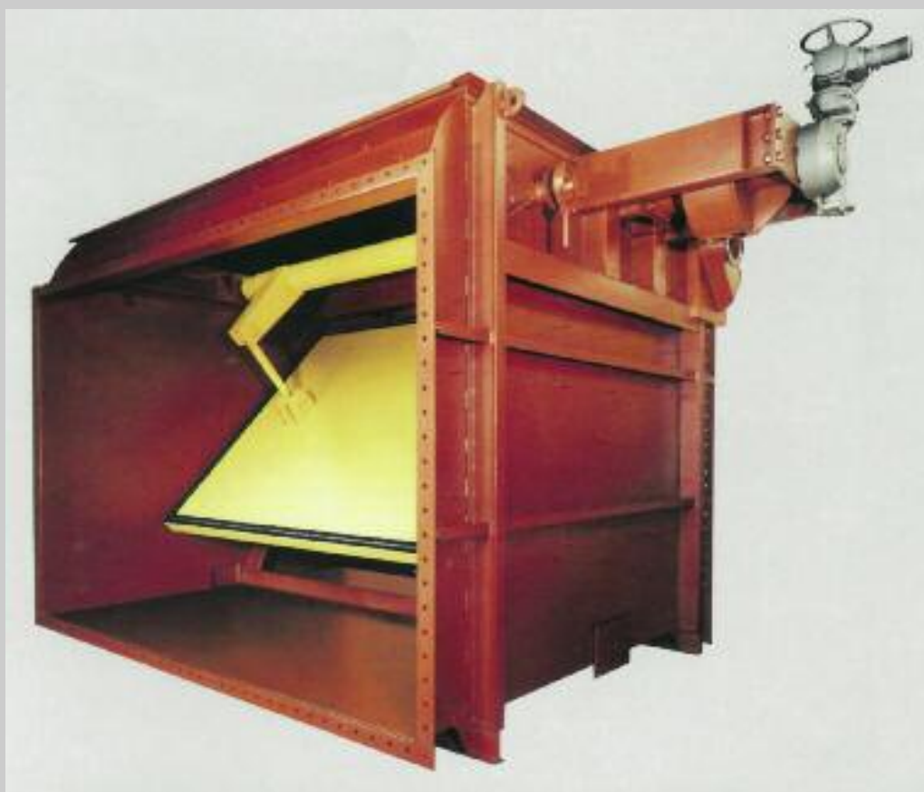
Gas diverter 4800 x 5300 mm, supplied for the FDG at the WESER power station, Veltheim BRD. Built-in scrubber. Drive via toggle. With double sealing and purge air, 100% leak-tight shut-off.
