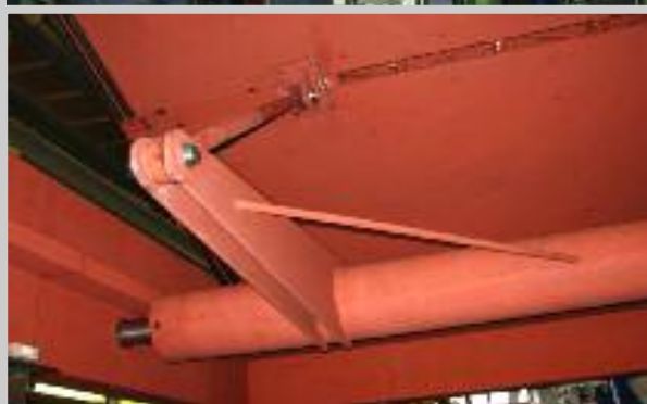
Illustration above: Flap damper NS 7480 x 5300 mm. Supplied for the De-NOx plant at the AMER power station in Holland. The lattice supported blade is driven via a toggle system (insert). 100% gas-tight using the NICROFLEX-HIPERFORM sealing system.
