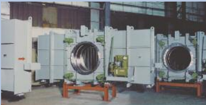
Illustration above: Goggle valve for installation in a vertical pipeline. The same execution is also deployed for vertical installation in a horizontal pipeline.
