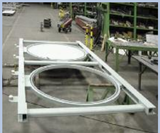
Illustration below: Goggle valve NS 2200, mechanically actuated during assembly in the factory
