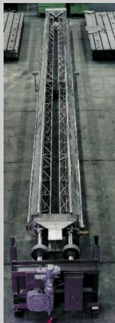
Picture on the right and left: Patented shut-off and gas modulation system, ND 600 x 17500 mm, for the combined cycle power station at Bitterfeld. This damper serves to either shut-off the integrated boiler bypass or for gas flow modulation towards it. Covering a blade span of 17500 mm was made possible by using the new, patented lattice structure supported blade design. The blades are made up of 17500 mm long latticed girders upon which free floating cover plates are fitted. The NICROFLEX-HIPERFORM seals high resilience guarantee a tight closure of the blades. In open position and high velocity, high temperature gas flow, the suitably stabilised sealing elements permit trouble free modulating operations. The system operates at temperatures of up to 700 degrees C . Even at such conditions no blade distortion has been observed.
