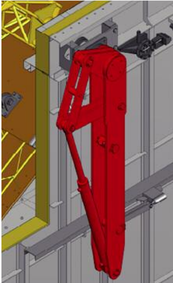
Picture below: dual toggle lever actuation arrangement for a DIVERTER, ND 5600 x 5600 mm
