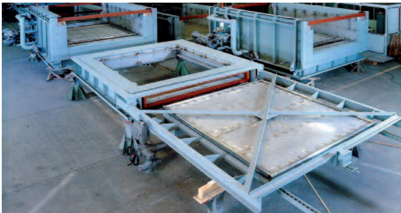
Picture above: Blanking plate guillotine, ND 3050 x 3050 mm for the Entek power station.
