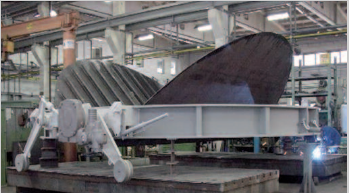
Picture above: Stack damper, ND 7000 mm dia supplied to BALKCE-DÜRR, Austria for the HRSG unit at Kastroe plant, Norway.
