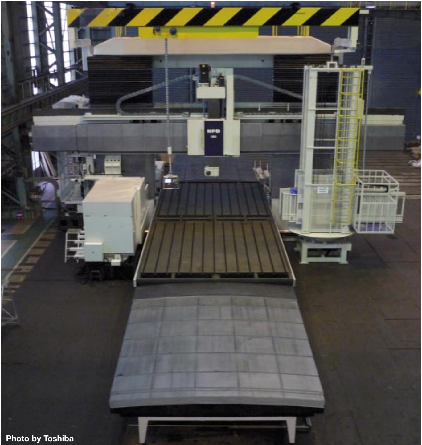
TOSHIBA -universal boring mill mit with telescopic covers supplied by RAUMAG-JANICH .
