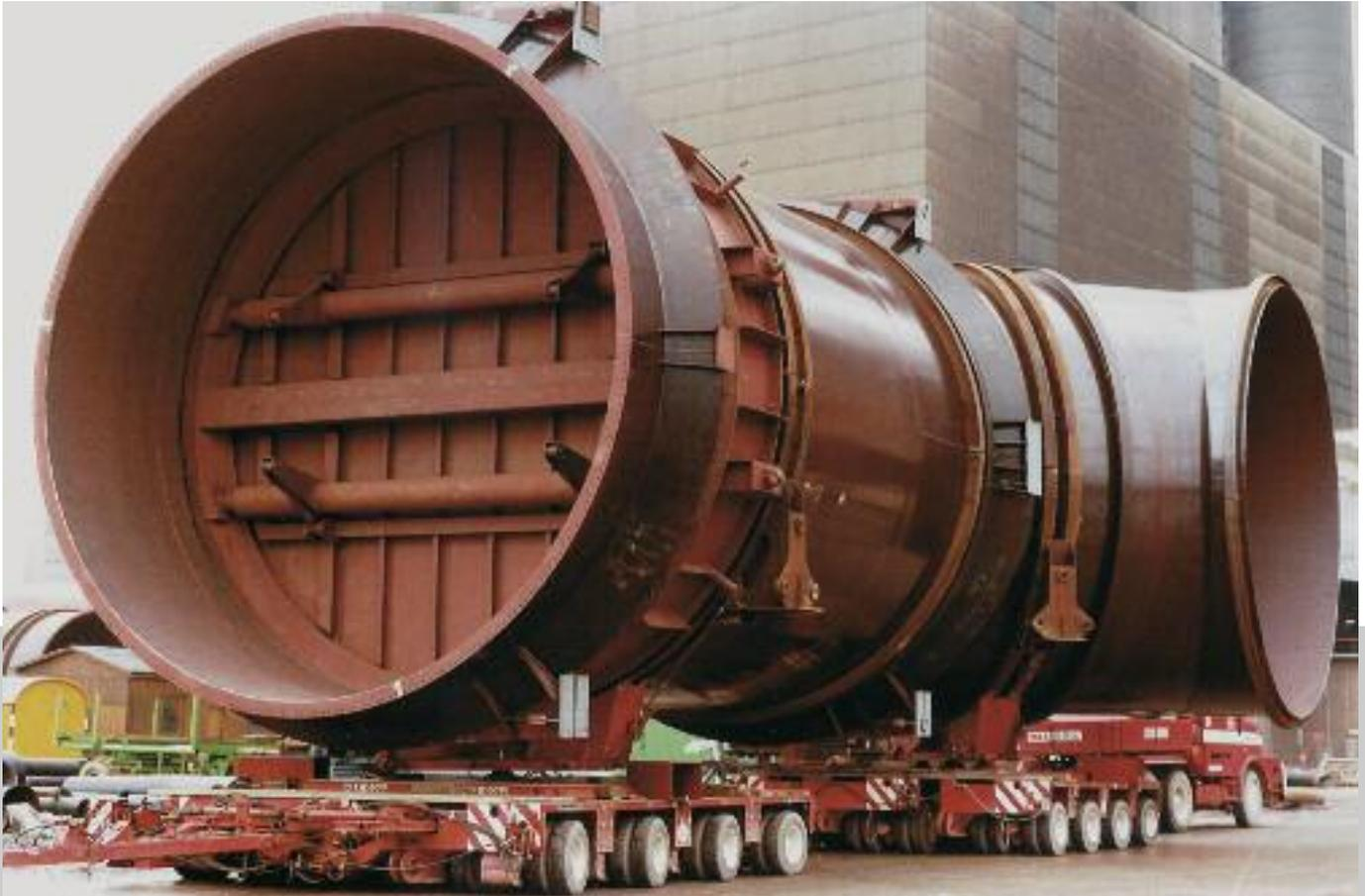
Illustration above: Flap damper DW 7000 mm with duct piece during transportation to the installation site.
