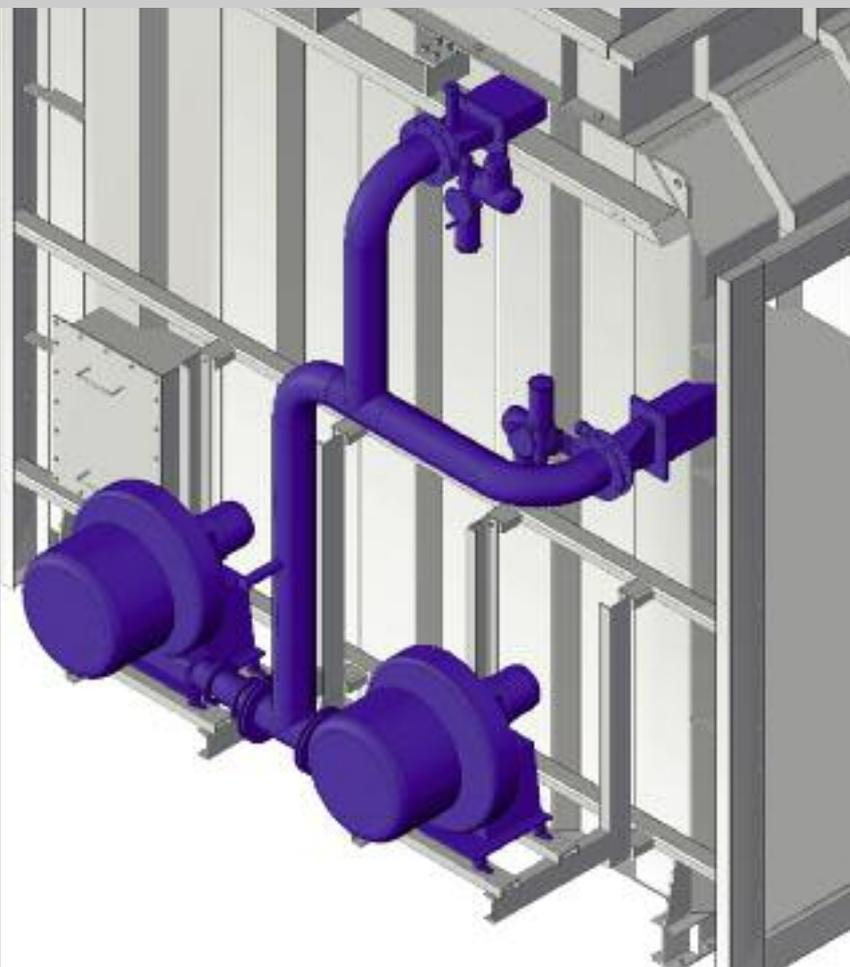
In conjunction with a double seal, a 100% shut-off of the hot gas flow is achieved by the introduction of purge air between the two sealing planes when the damper blade is closed. In the process, the purge air pressure must be greater than the pressure of the gas being shut off.
