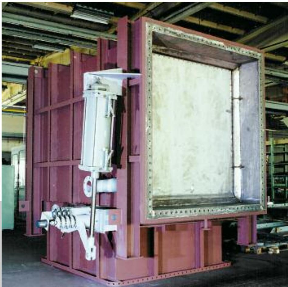
**Gas diverter 2300 x 2300 mm** supplied through **Noell-KRC** for the **FDG** at the **Amsdorf BRD power station**.
